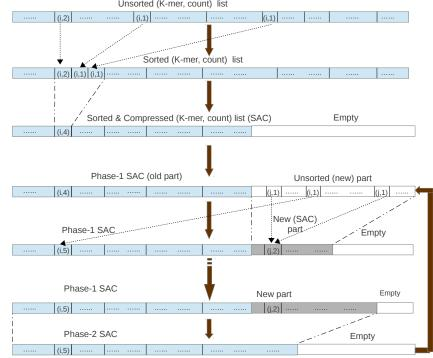
Fig. 1. The Sorting and compaction mechanism. We start with an unsorted k-mer array. It is sorted and compacted (Phase-0 SAC). The empty part is filled with unsorted k-mers, sorted and compacted. After repeating this step several times, the compacted new part almost fills up the whole array. Then all items are sorted and compacted to produce Phase-1 SAC. This cycle repeats until all k-mers have been seen. Unsorted (K-mer, count) list
